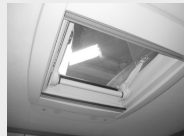
Fig. 31: Tagluge 400 x 400 mm VisionStar 700 x 500 mm
