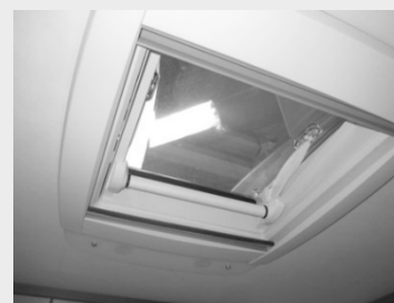
Afb. 49: Dakluik 400x400 mm VisionStar 700x500 mm
