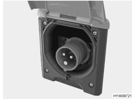
Fig. 69 230 V connection on the vehicle (CEE socket outlet)
