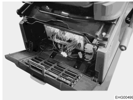
Fig. 65 Position of the transformer/rectifier
